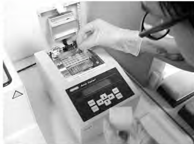
Samples are run through PCR, 40 cycles of basic denaturing and annealing stages.
