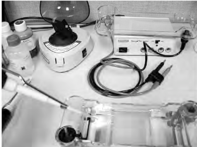
Samples are loaded into electrophoresis wells, along with molecular ruler and controls.
